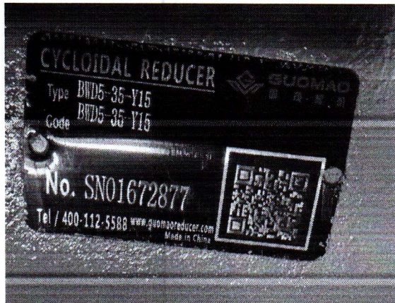
No. 17 - Cycloidal Geared Motor for Sludge, Slurry Mixer. IP55F-380V, 变频电机 50HZ nameplate
