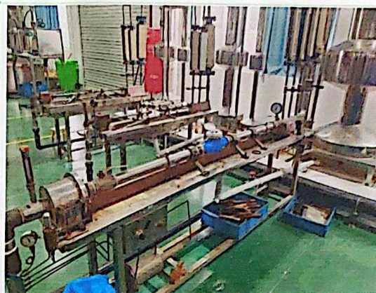
Fig 20. Static hydraulic pressure test
