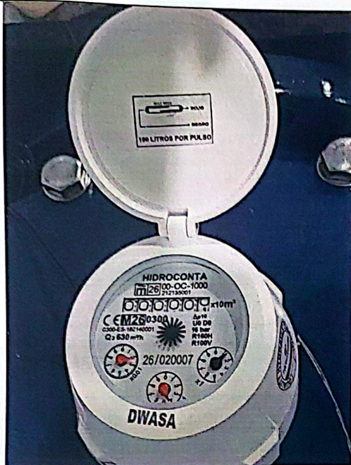
Marking – water meter DN200
