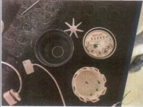
Disassembled mechanism of water meter
